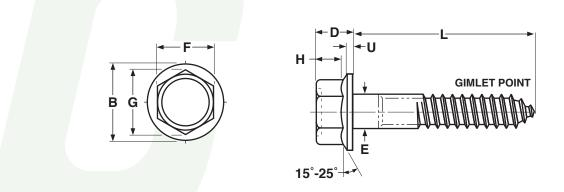
Length of a hex flange lag screw (L) is measured from the underhead bearing surface to the extreme end of the screw. Minimum thread length is 1/2 length of the screw plus 0.50 inch or 6 inches, whichever is shorter.
